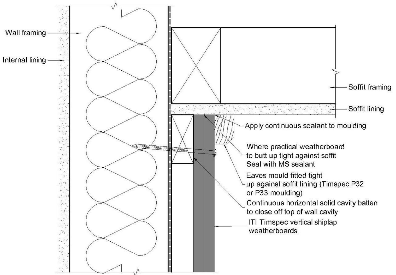
VC 601 Roof/ Wall Top Plate – Flat Soffit
