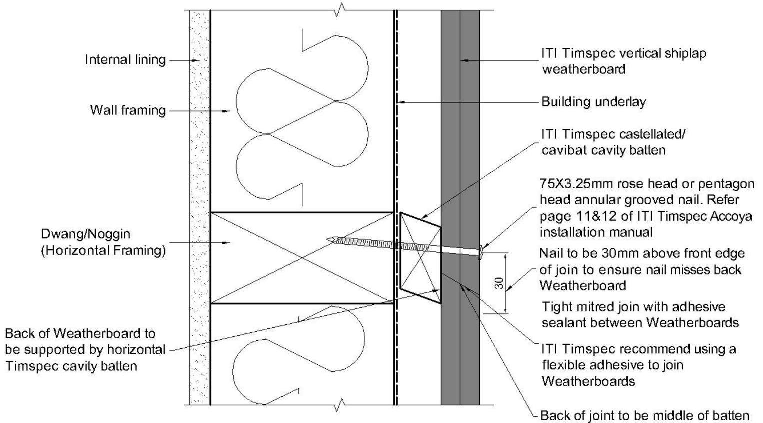
**VC 402 Within Board Joint – Scarf Joint**
