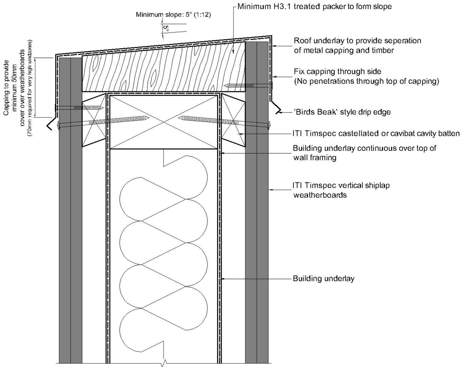
**VC 701 Parapet Capping Expansion Joint**
