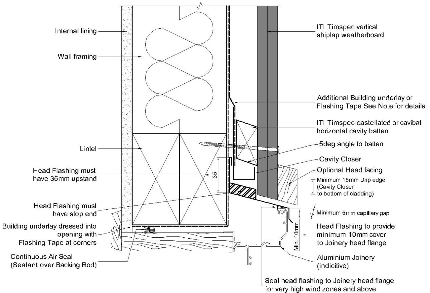
Note: Additional Building underlay to extend up wall to nearest lap above and extend down as far as possible into Cavity Closer.
