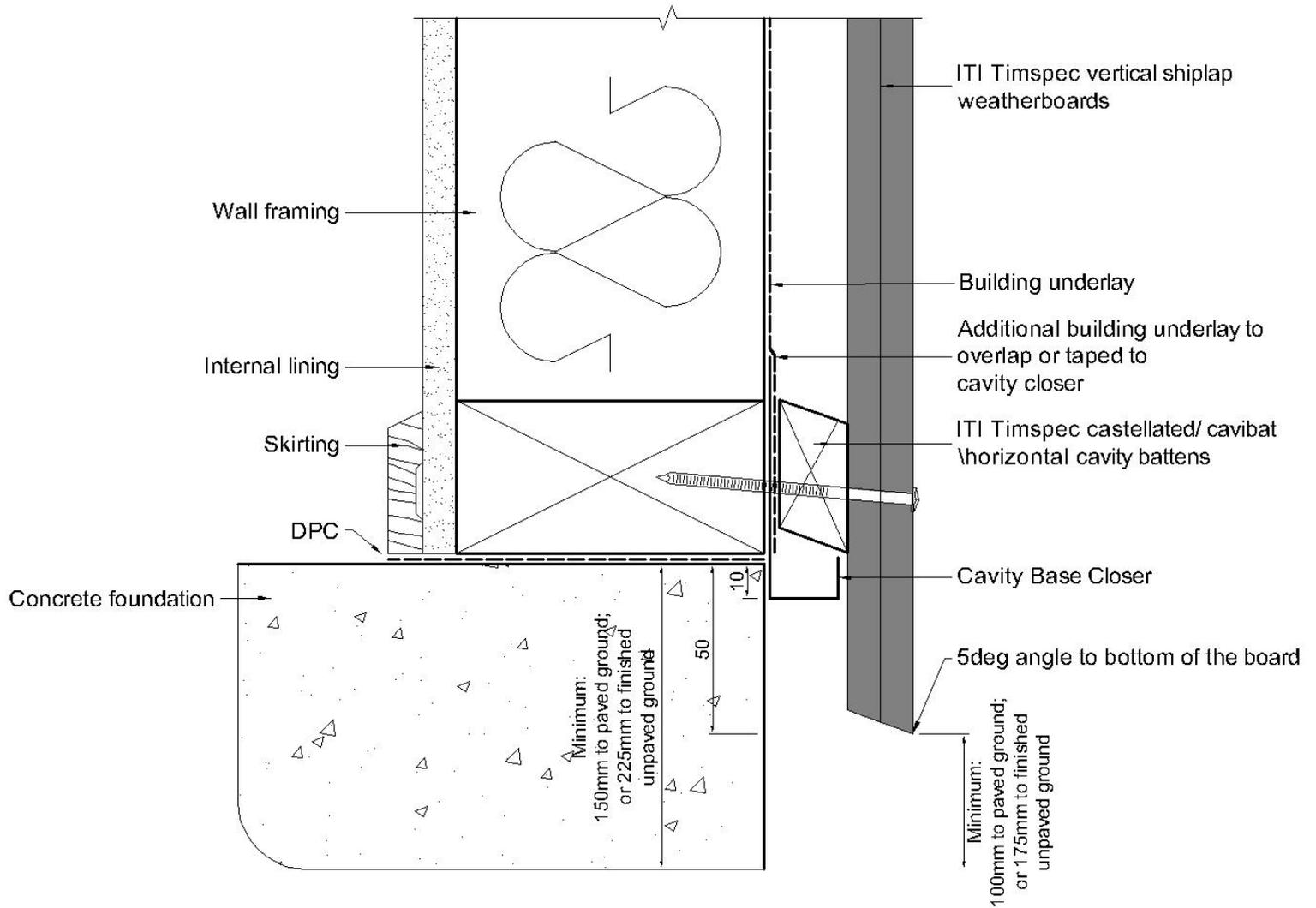
VC 501 Base, Concrete Slab on Ground
