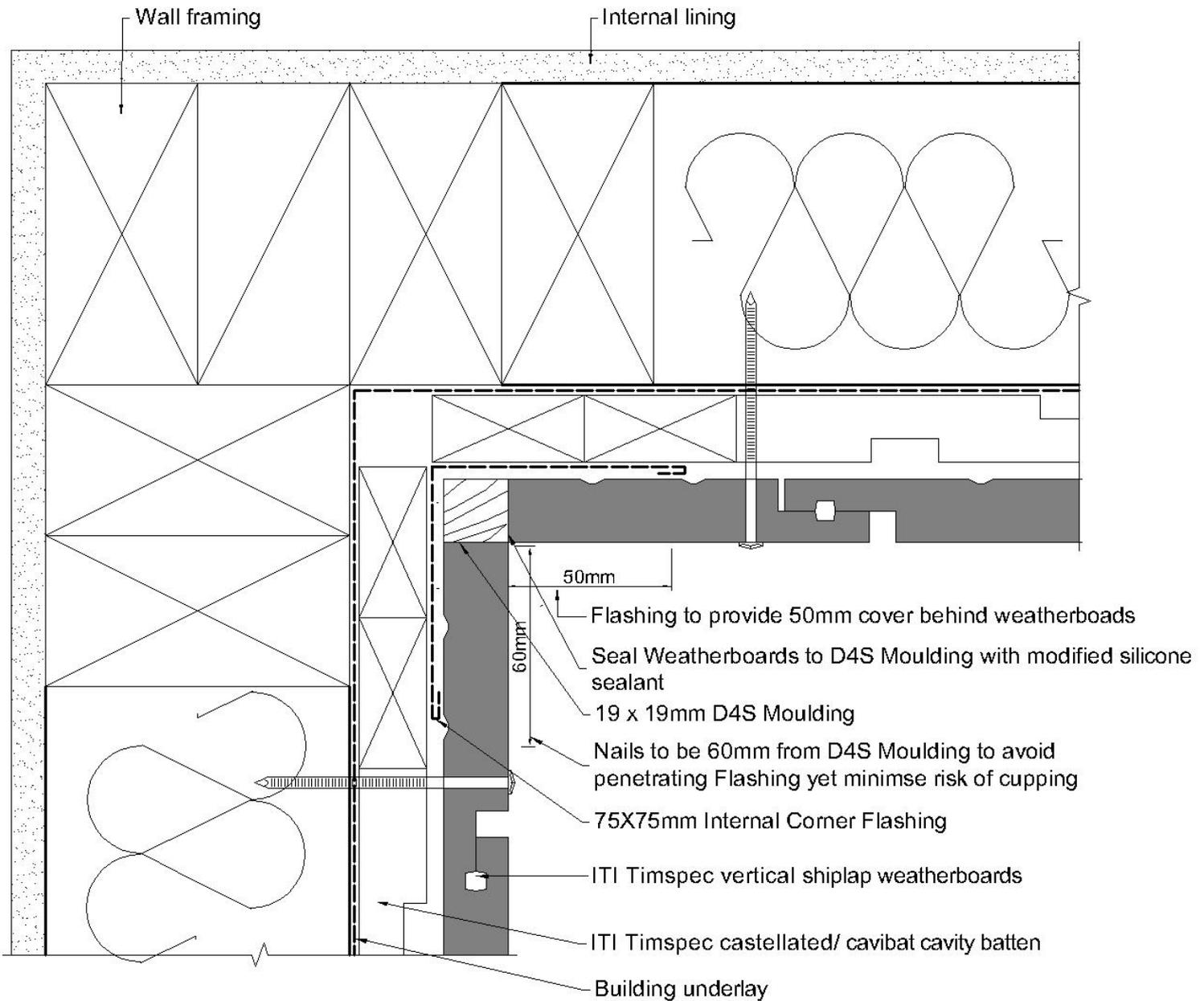
**VC 300 Internal Corner - 19X19mm Corner Moulding**
