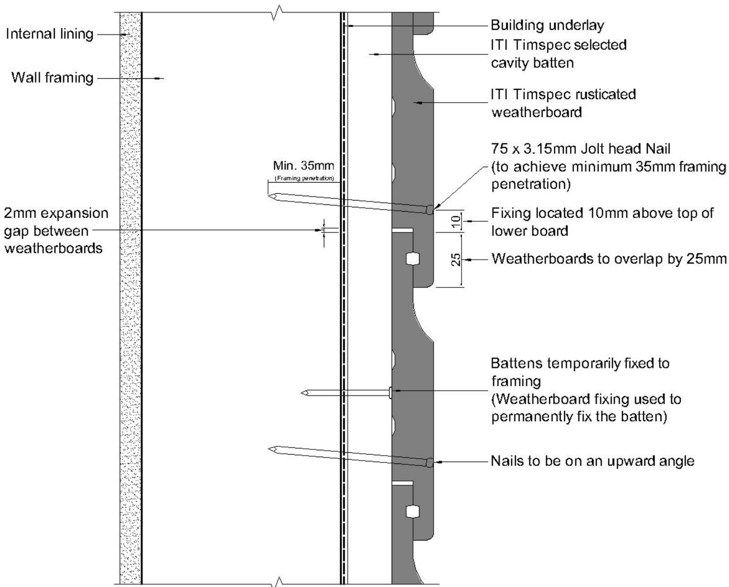
**FIGURE 13. 2 RC 106 STAIN FINISH WEATHERBOARD WITH STANDARD CAVITY FIX**
