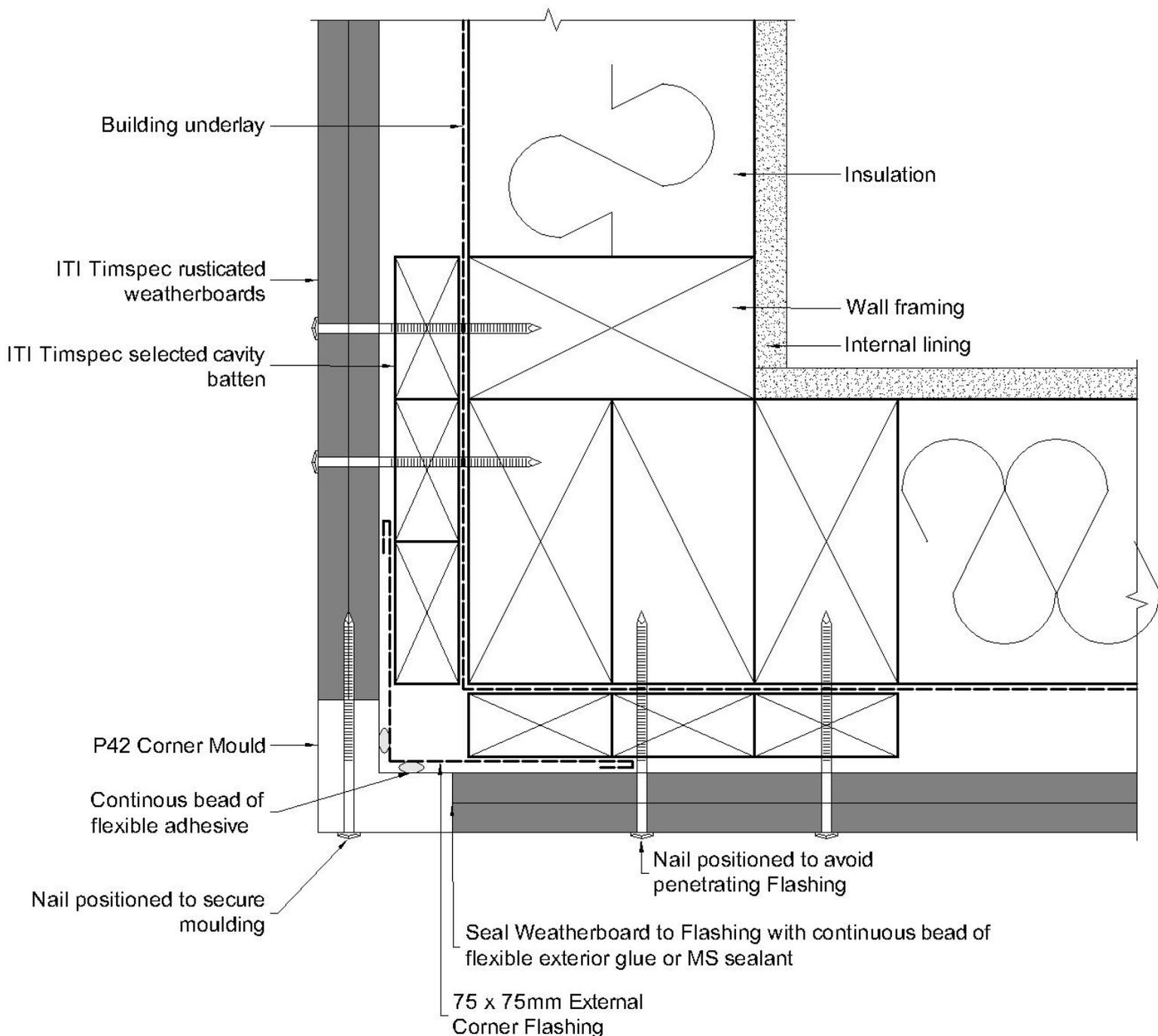
**FIGURE 13. 13 RC 406 EXTERNAL CORNER – P40 CORNER MOULDING**
