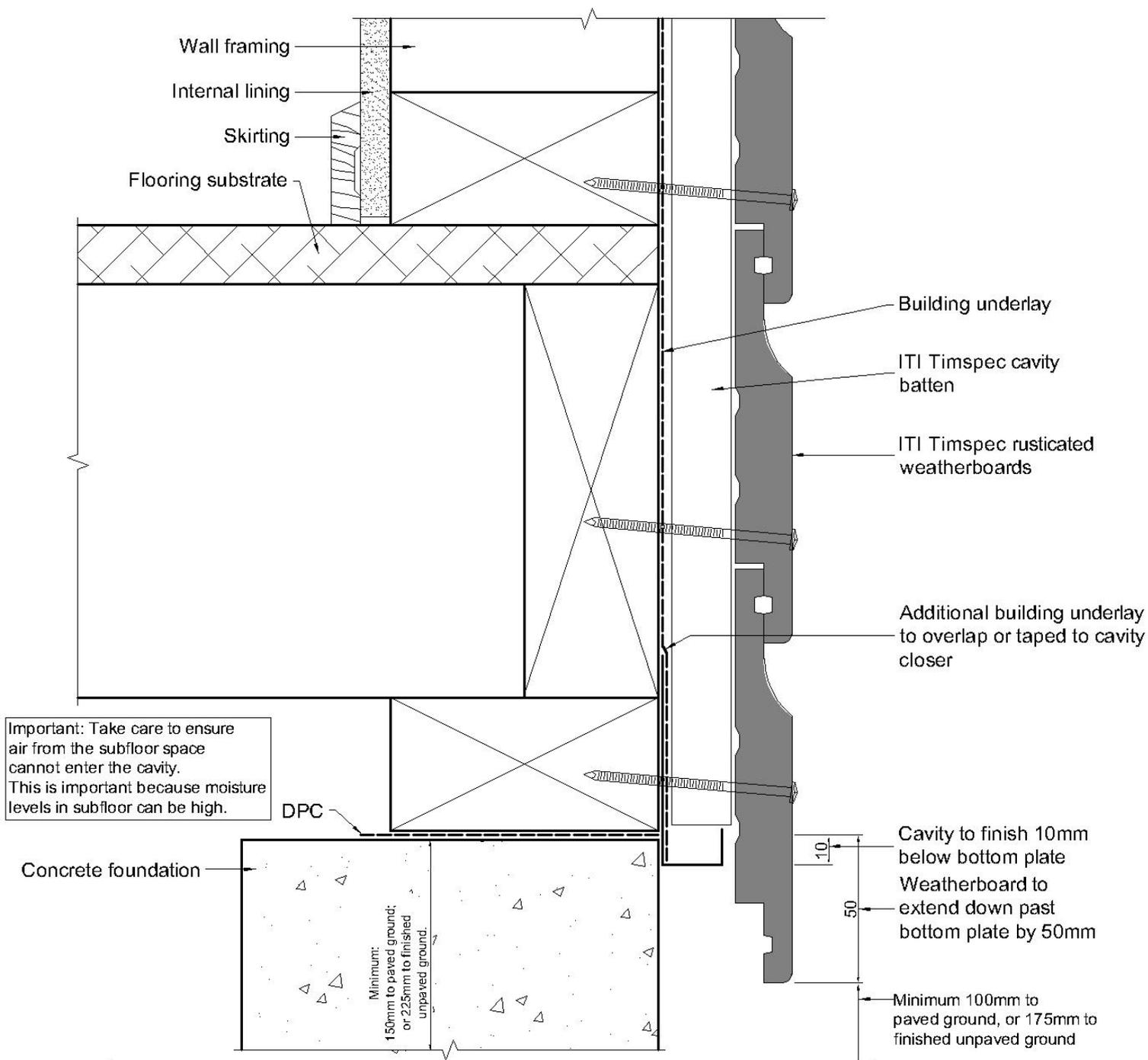
**FIGURE 13. 16 RC 503 BASE, CLADDING FINISH ABOVE DECK**
