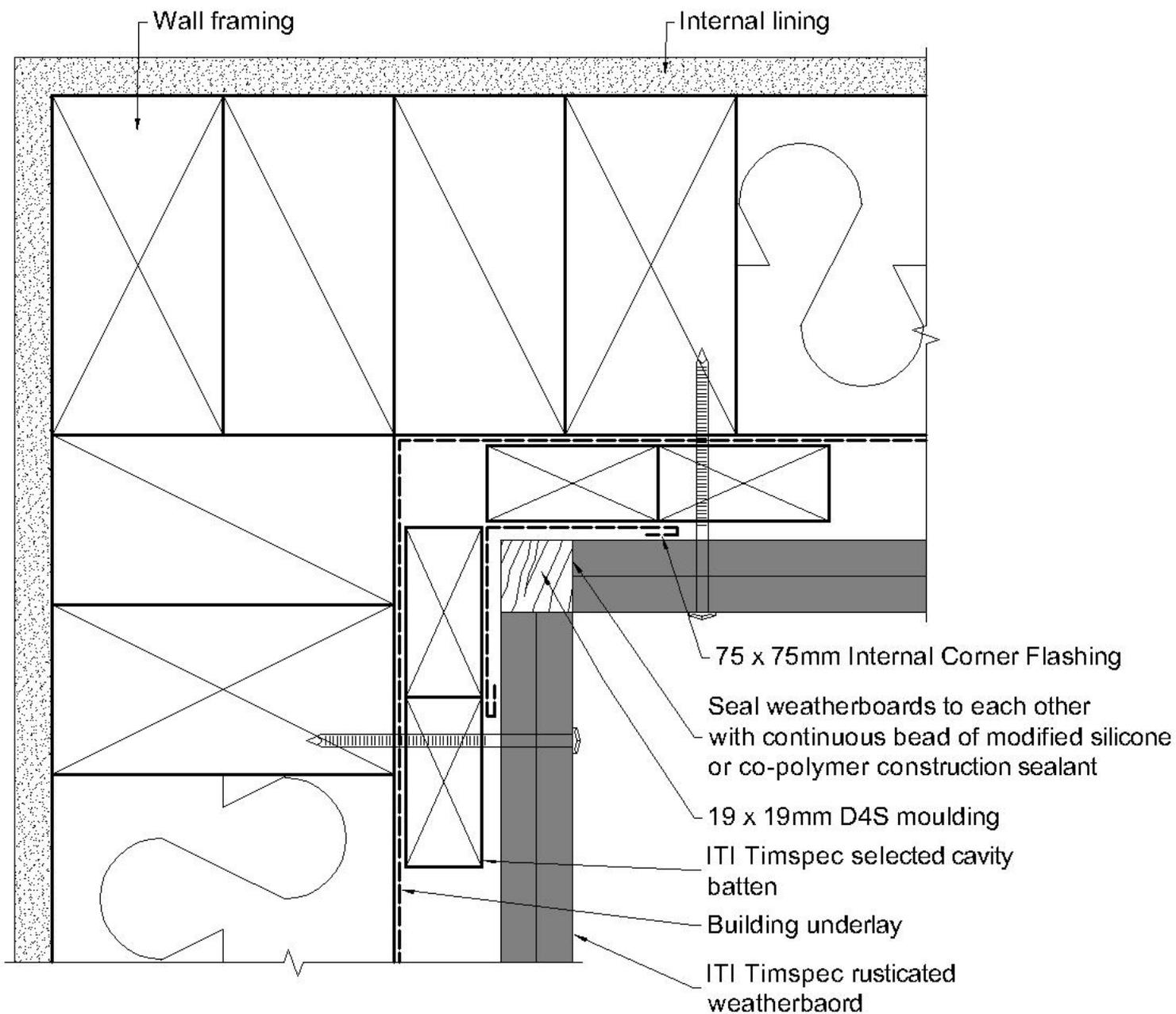
**FIGURE 13. 7 RC 301 INTERNAL CORNER – 40X40MM MOULDING**
