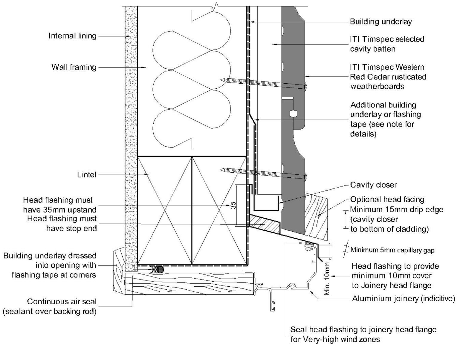
Note: Additional building wrap to extend up wall to nearest lap above and extend down as far as possible into cavity closer.
