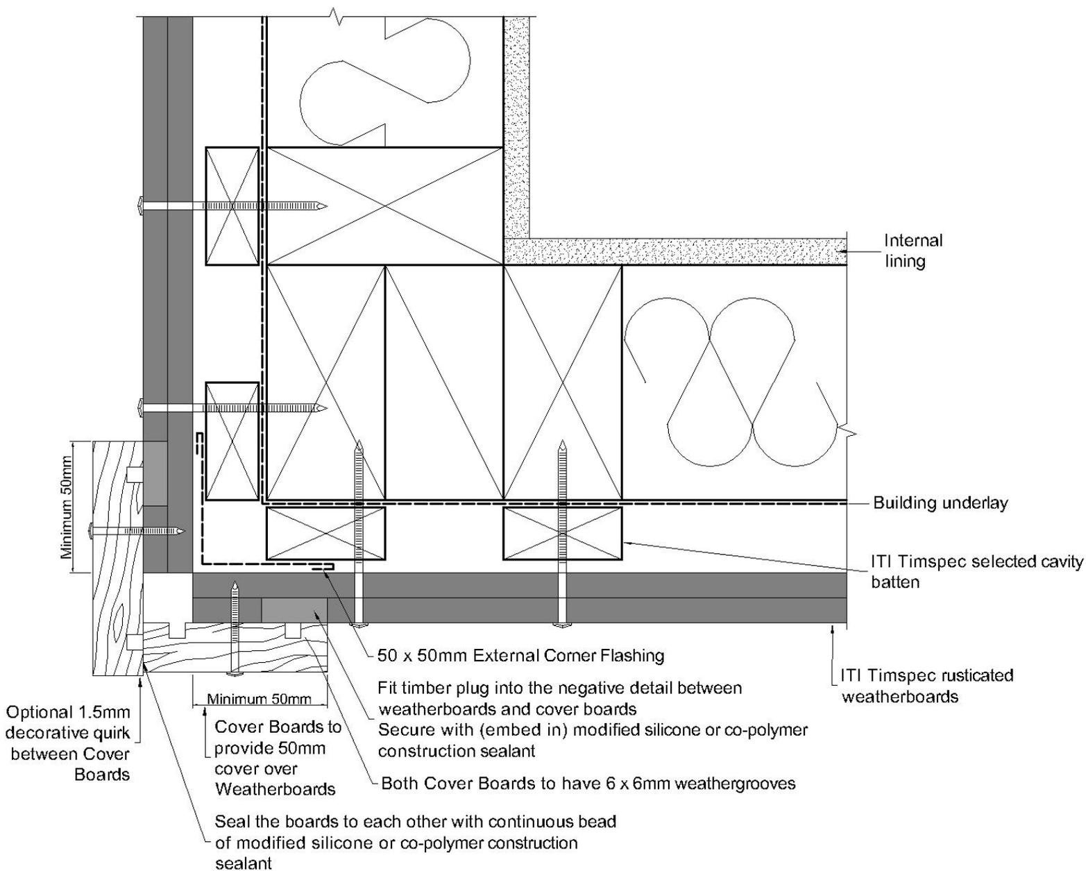
**FIGURE 13. 12 RC 404 EXTERNAL CORNER – P42 CORNER MOULDING**
