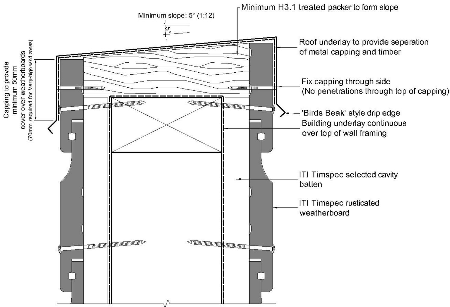
**FIGURE 13. 20 RC 702 BALUSTRADE, INTERSECTION WITH WALL**
