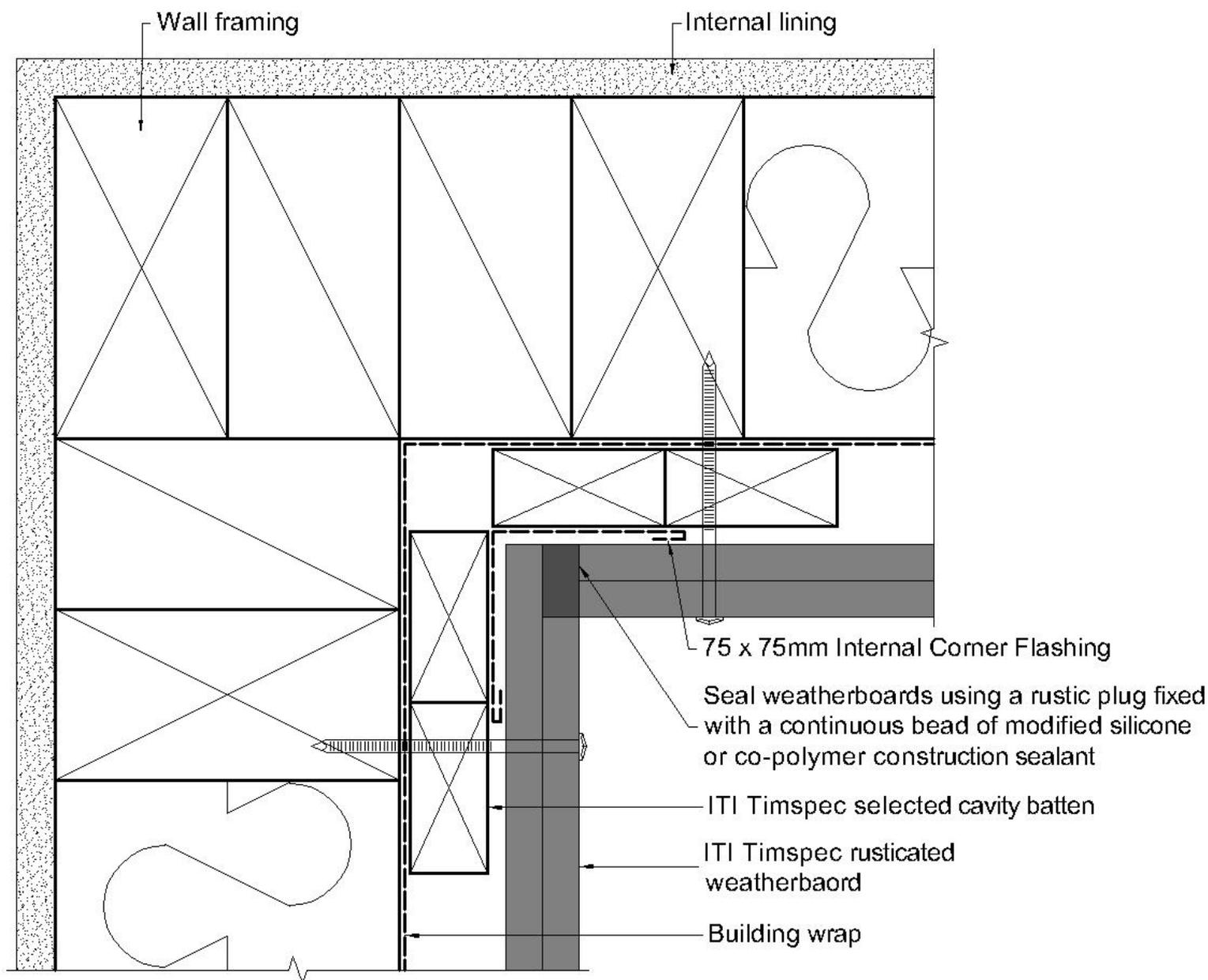
**FIGURE 13. 9 RC 401 INTER-STOREY JUNCTION**
