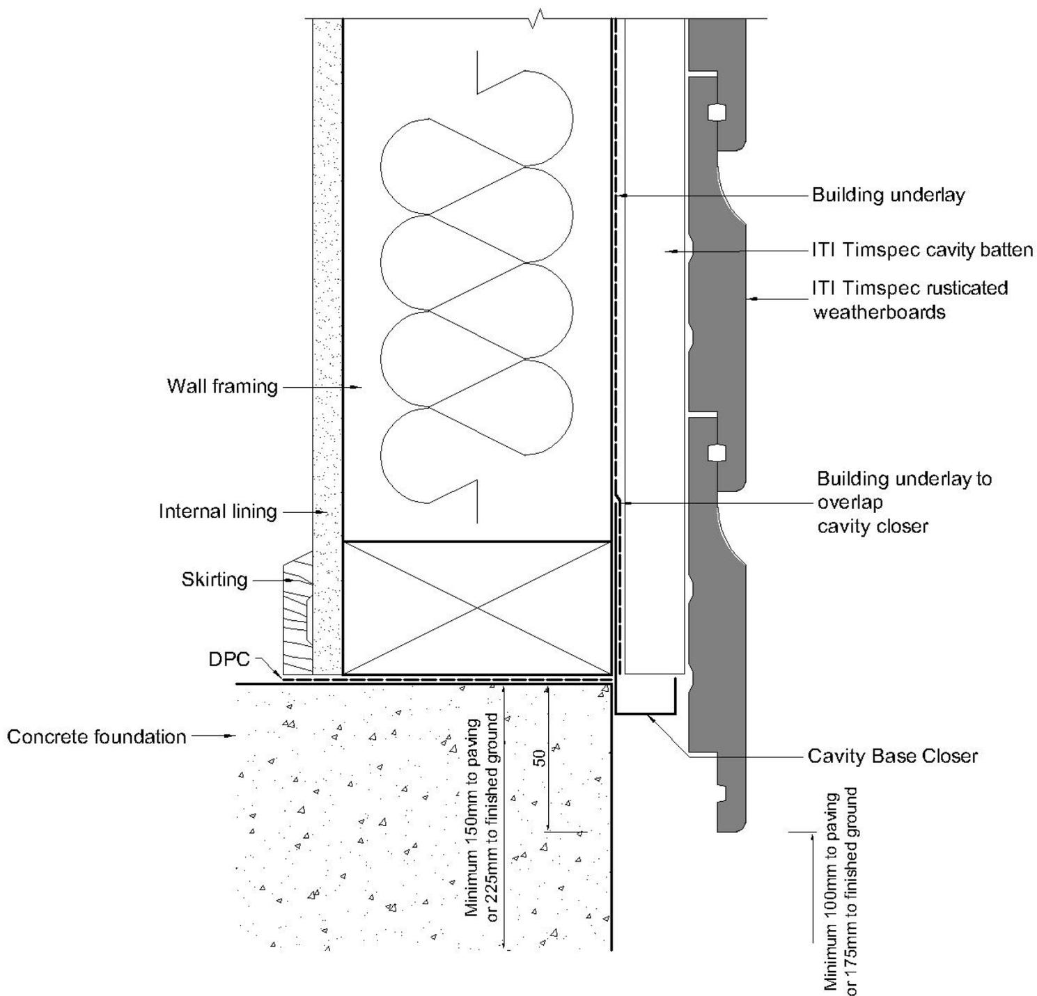
**FIGURE 13. 15 RC 502 BASE, TIMBER FLOOR**
